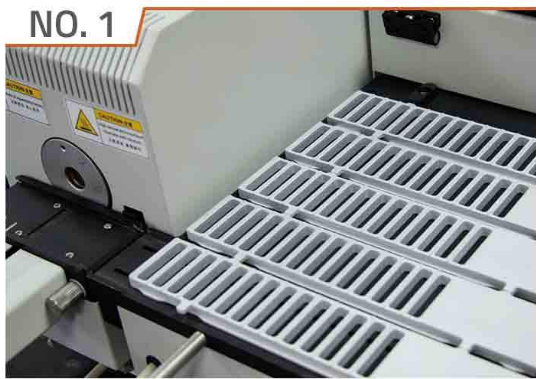
NO. 1 70 position auto-sampler for high sample throughput
